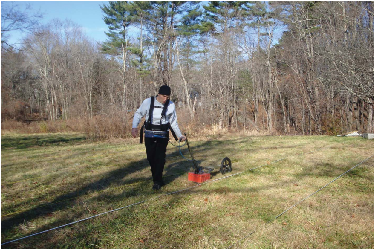
Gutbrod 2011 400 Megahertz (MHz) antenna and survey wheel
