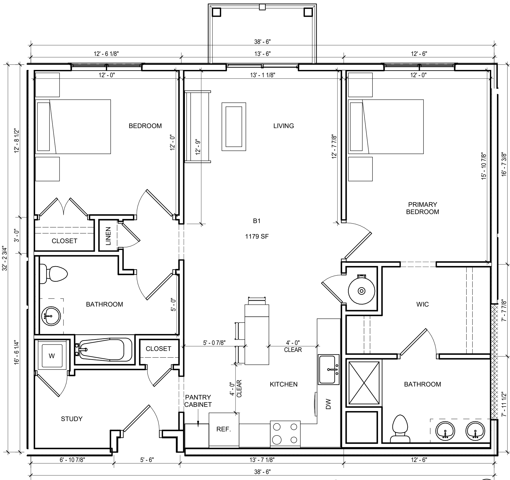
ENLARGED UNIT PLAN - 2 BED - B1
